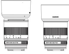
Align the attachment reference point on the hood with the reference point for a hood on the lens, push the hood onto the lens and turn the hood clockwise until it makes a clicking sound.
